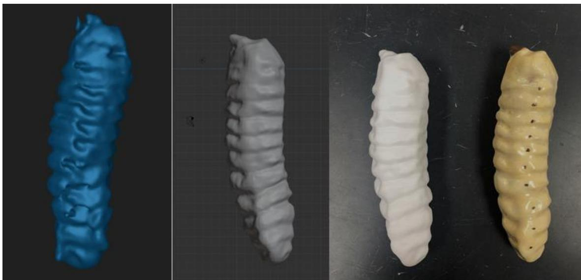
**Figure 4.** Creation process for the beetle larva of a roundheaded borer 3D print. Left to right - initial scan image and data (Revoscan 5 software), finished digital file after cleanup and detail sculpting (Blender software), unpainted print of the model, and the final print after sanding, painting, and sealing. Note that the sealing process gives a shiny appearance to the model. All images by author, 2024.
