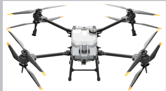
Fig. 1. The DJI AGRAS T40 weighs 110 lbs and is 9 ft x 10 ft.
