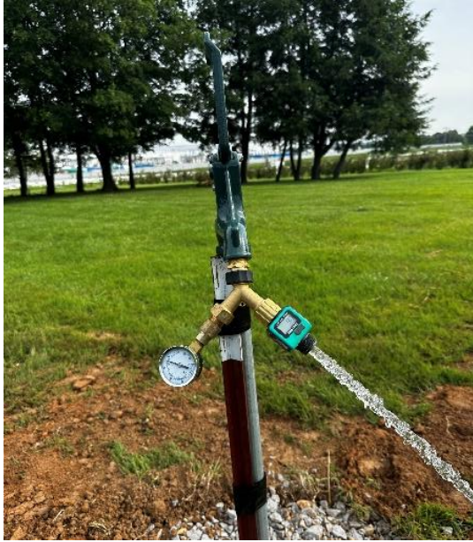
Figure 1: Method of measuring flowrate (right side of splitter) and pressure (left side of splitter) of a water source.
